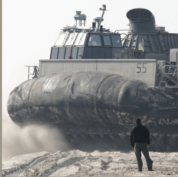
AEF pioneered the production of hovercraft skirts made from natural rubber neoprene.
