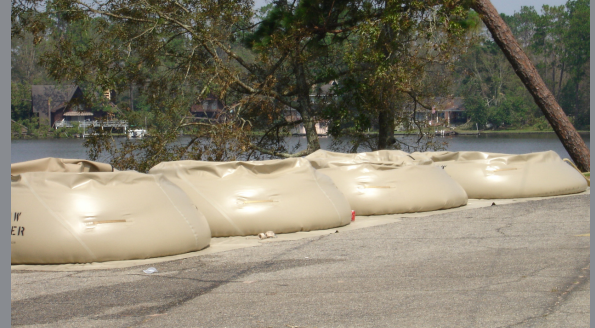
AEF onion tanks deployed after Hurricane Katrina
